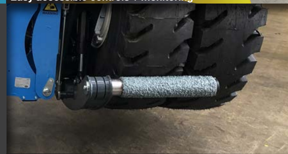
Stone-coated pipes ensure a safe grip
