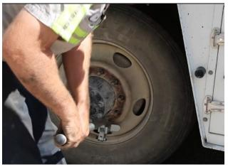
4. Insert the heavy duty wheel puller hooks into the opposite side and repeat procedure. Repeat steps 2&3 till the tire is removed.
