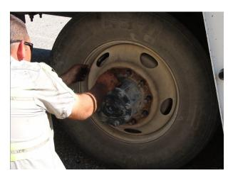
1. Screw a set of lug nuts on opposite sides of the tire to protect the wheel stud.
