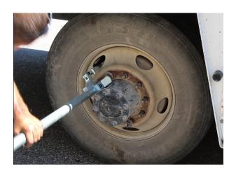
3. Apply pressure to level to loosen wheel off hub.
