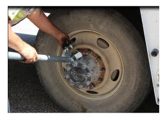
2. Insert the heavy duty wheel puller hooks into the rim and brace the heel of the tool against the center hub.
