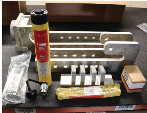
2. Remove Rubber Cap covering threads on the Hydraulic Cylinder (Part #9). 3. Remove Cap on top of the Hydraulic Cylinder (Part #9). Remove Saddle by twisting out to expose threads.
