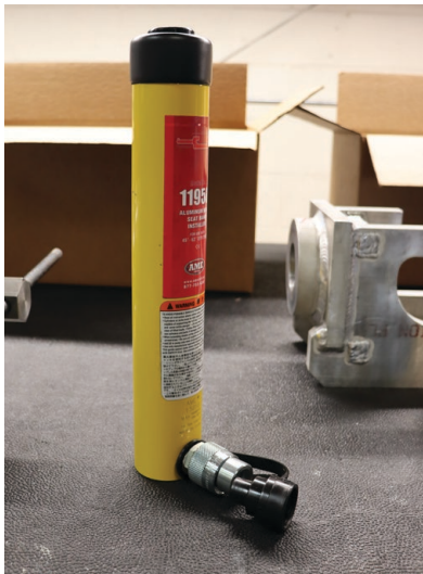
2. Remove Rubber Cap covering threads on the Hydraulic Cylinder (Part #9). 3. Remove Cap on top of the Hydraulic Cylinder (Part #9). Remove Saddle by twisting out to expose threads.
