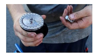
**Step 9.** Slide wheel into the hole and hand tighten the bolt/washer to the jack.
