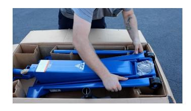
**Step 7.** Pull rear end of jack out of the box and rest on the side of the box.
