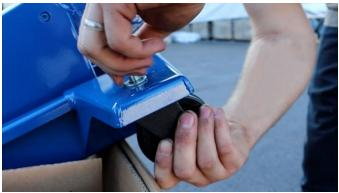
**Step 10.** Hold the wheel in place and using your hand drill and 19 mm socket, tighten the bolt to the jack.
