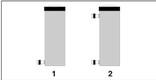
**IMPORTANT:** Double-acting cylinders must have both couplers connected.
