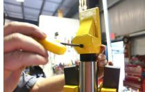
Remove set screw in order to remove the plunger.
