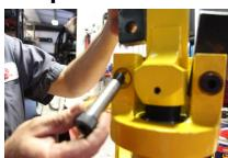
Remove bolt with 3/8" allen wrench and 15/16" wrench for nut. Remove old claw and install longer claw. Re-tighten bolt. Repeat for the other side.
