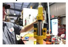
Thread on new plunger, tighten set screw, then retract the piston.
