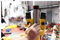
After removing the old plunger, confirm the threaded adapter is fully threaded into the piston.
